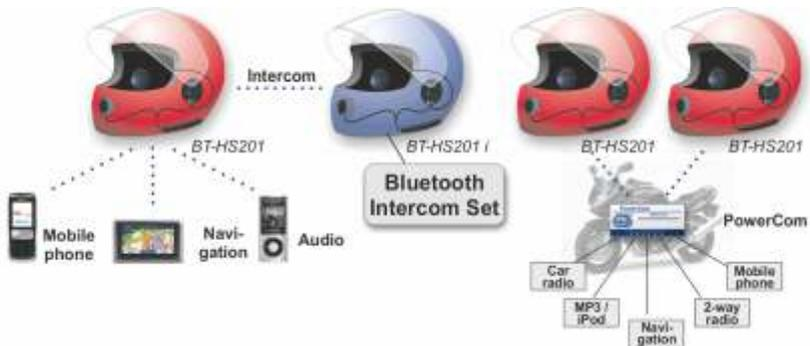
The Stealth Bluetooth Helmet Set 201 can be used with all Bluetooth devices that are compatible to A2DP, hands-free or headset profile, e.g. Bluetooth mobile phones, navigation systems, MP3 as well as with all motorbike communication systems of the **AKE PowerCom** series with Bluetooth to helmet.
